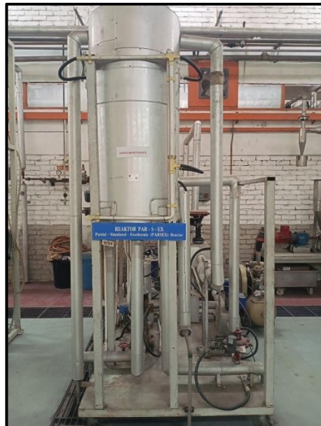
Figure 2. Partially Simulated Exothermic Reactor (UM)
